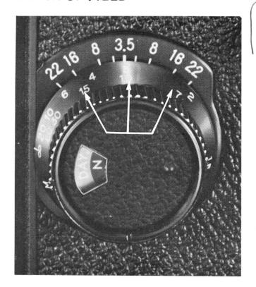
The depth of field for a given aperture and camera-to-subject distance can be read off the depth-of-field scale around the Focusing Knob. By checking this scale, you can easily determine before shooting the extent over which the objects will appear sharp and clear.
