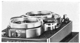
2 Center the desired shutter speed in the Shutter Speed Indicator Window by turning the Shutter Speed Control Dial. The exposure meter pointer in the Exposure Indicator Window is coupled to the shutter mechanism and will shift in either direction when the shutter speed is adjusted.
