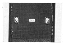
When loading a 120 film (12 exposures), hold the back cover with both hands and slide the Film Pressure Plate with your thumbs until it clicks into position and the sign 12 EX. (in green) appears in the window in the middle of the plate. When loading a 220 film (24 exposures), hold the back cover with both hands and slide the Film Pressure Plate with your thumbs until it clicks into position and the sign 24 EX. (in red) appears in the window in the middle of the plate.
