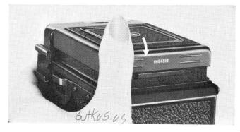
When the camera is to be left unused, fold the focusing hood. This will switch off the meter and prevent draining of battery power.
