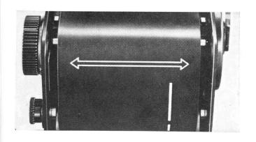
Tontinue winding the film until the "start" mark on the film leader paper lines up with the GREEN triangular (◄) "start" mark for 120 film.
