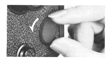
① Open the Battery Compartment Cover holding with finger and by turning it counter-clockwise. This camera uses a 1.3 V mercury battery to power its exposure meter. Use either Mallory PX-13B, Eveready EPX-13 or equivalent.
