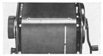
Tontinue winding the film until the "start" mark on the film leader paper lines up with the RED triangular (▶) "start" mark for 220 film.
