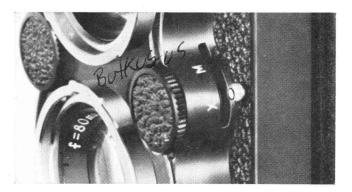
Switch the Flash Synchronizer Selector to "X" when using F-class flash bulbs or electronic flash.
