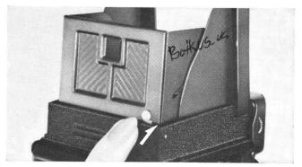
To close the Cover, push the Release Button on the back of the Focusing Hood.
