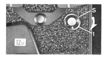
The letter "S" appears in the Exposure Counter during the film loading operation. After closing the Back Cover, wind the crand-handle until the figure "1" appears in the Exposure Counter Window.
