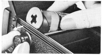
3 Pull out the Upper Spool Holder Knob and take out the exposed film from the film chamber. Paste the seal to prevent recoiling and wrap the film in light-proof paper.
