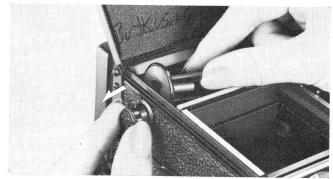
2 Pull out the Upper Spool Holder Knob and place the empty spool in the Take-Up Spool Chamber. After the Take-up Spool is set properly in the camera, return the Spool Holder Knob to its original position.
