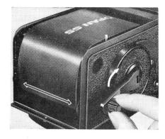
4 Place the new roll of film in the lower film chamber while pulling out the Lower Spool Holder Knob. Also make sure that the Lower Spool Holder is returned to its original position after loading the film.
