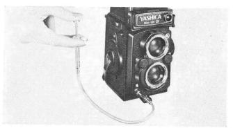
When shooting at 1/30 sec. or slower shutter speeds or making B (bulb) exposures, it is advisable to mount the camera on a tripod and to use a cable release to prevent erratic movement of the camera during exposure. To mount the cable release, screw it into the Cable Release Socket on the Shutter Release Button.
