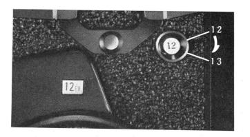
1 When the figure "12" appears in the exposure counter window, it signifies that the full length of the film has been exposed. Another wind of the crankhandle will set the exposure counter between "12" and "13", but continue winding until the crank-handle turns freely without tension.
