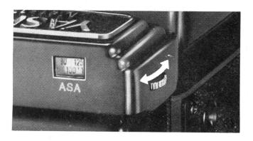
1 Turn the ASA Film Speed Setting Wheel until the figure denoting the ASA rating of the film in use aligns with the red indicator in the ASA Film Speed Indicator Window.
