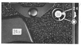
When the figure "24" appears in the exposure counter window, it signifies that the full length of the film has been exposed. Another wind of the crank-handle will bring out the ● mark in the window, but continue winding until the crankhandle turns freely without tension.
