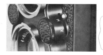
Always set the Flash Synchronizer Selector to "M" with M-class bulbs.
